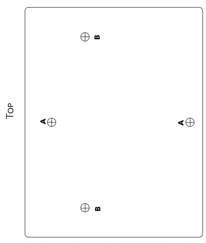
Remove this page with scissors or make a copy. Line up the template so the holes marked "A" are centered on a stud and tape it to the wall. Screw in a  $\#12 \times 2$ " wood screw (included in the manual packet) in both holes marked "A", leaving an 1/8" gap between the wall and the screw head. Remove the template and hang the controller over the 2 screw heads. If a stud cannot be located it will be necessary to use four 1/4" x 2" molly bolts in the holes marked "A" and "B".
