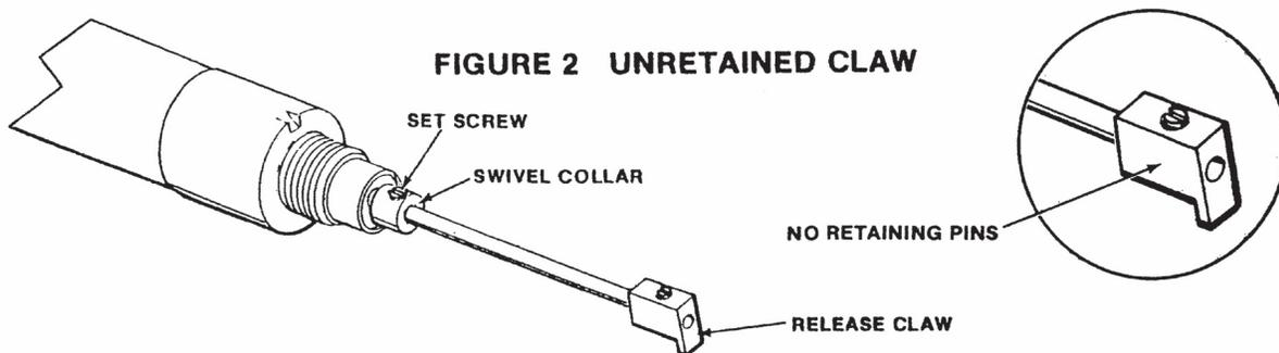
**NOTE:** The tube assemblies depicted in the above diagrams are "P" style; however, the directions apply to all KILN SITTER models. In addition, the release claw is not a part of the tube assembly replacement part.
