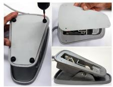
1. Unscrew the 4 feet using a Philips screwdriver. Then remove the plastic cover and make sure the foot pedal is in the STOP position. Turn the power ON.
