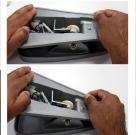
5. Push the pedal back and forth to test the START and STOP position of the potentiomter.
