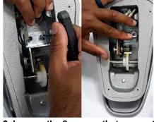
2. Loosen the 2 screws that connect the potentiometer (POT) to the bracket to the foot pedal housing. Separate the POT (silver gear) from the white plastic gear so they are not touching.
