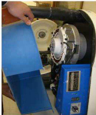
1.Remove the undercover by removing all undercover screws then sliding the undercover off.
