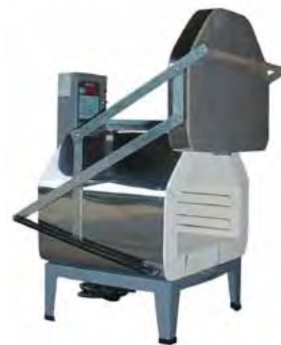
1818FLE 17.5" x 18" d x 12" h @ peak Shown with Guillotine Lift Option
