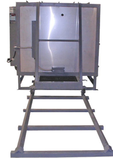
Custom FL78E 60 cubic feet Car Kiln
